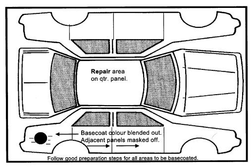
Apply basecoat color to spot repair and blend out.
